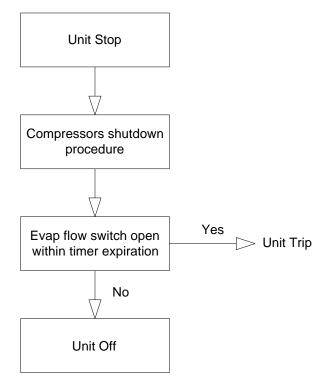
Fig. 18 – Unit shutdown sequence
