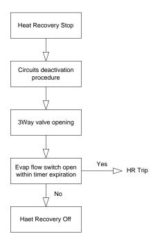
Fig. 20 – Heat recovery shutdown sequence
