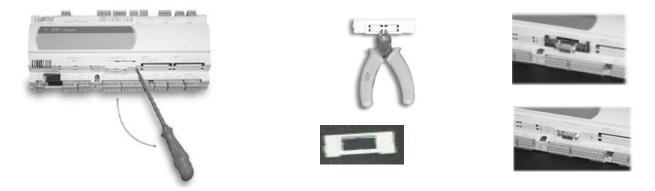
As per the pictures above, to properly plug-in the card, open the cover of the serial card plug at the bottom of the controller, securely plug-in the card and close it back.
