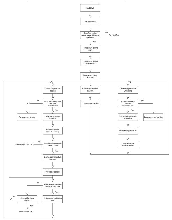
Fig. 17 – Unit startup sequence
