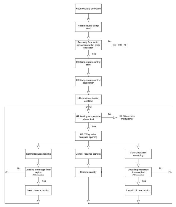
Fig. 19 – Heat recovery startup sequence
