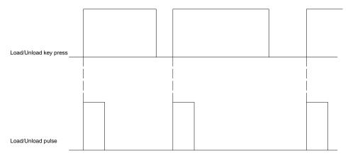
Fig. 13 – Compressor manual control
