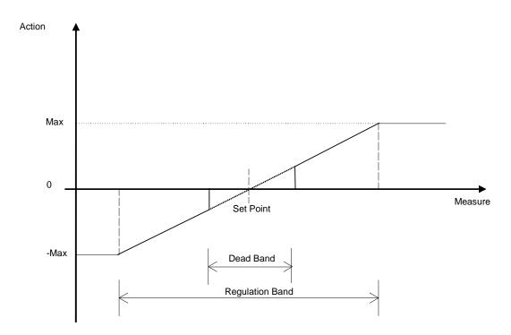
Fig. 12 – PD controller proportional action
