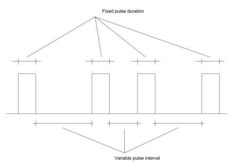
Fig. 11 – Loading or unloading pulses
